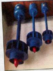
Fig. 32: Phillipines, Pico-Hydro Power, Propeller Type Turbine
